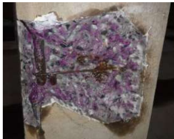
Figure 15 Concrete broken out and tested for pH with phenolphthalein
