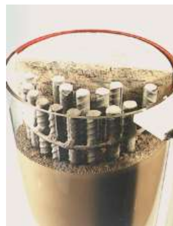
Figure 2: Cross-sectional view of fluid micro-concrete repair mortar
