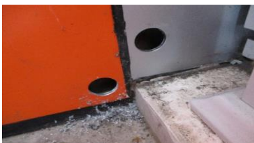
Test sampling to check ACP composition
